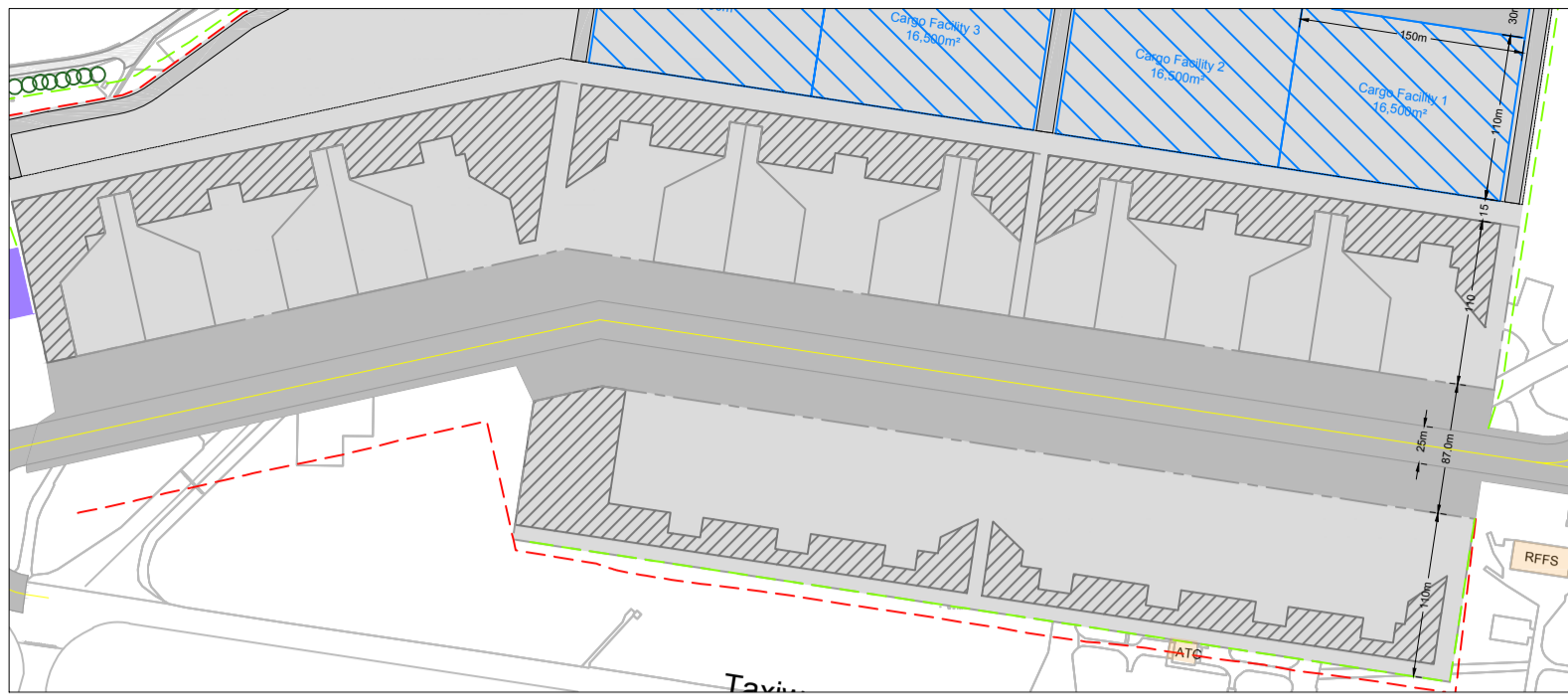
Code F Aircraft Configuration (6 positions) Scale 1:5000
